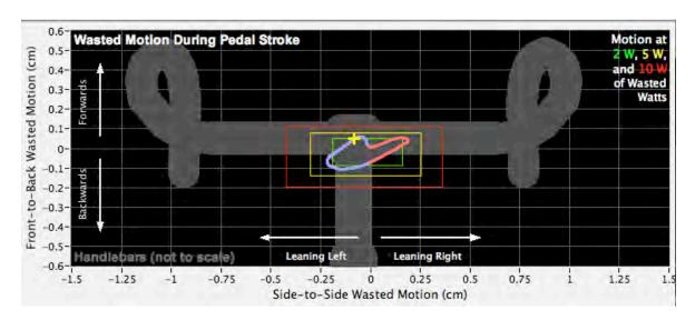
The Wasted Motion Plot shows the motion of the bike, relative to the center of mass of the rider, both side to side, and front to back, as the cyclist pedals through a complete turn of the crank.
