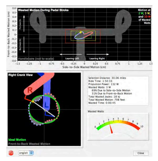
**NOTE**: IN THE "WASTED MOTION" PLOT AND "RIGHT CRANK" PLOT, RIGHT STROKE INFORMATION IS COLORED IN PINK. LEFT STROKE INFORMATION IS COLORED IN LIGHT BLUE.
