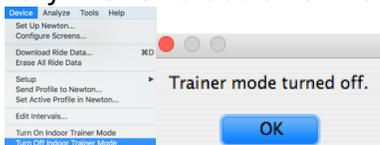
7. IMPORTANT: WHEN INDOOR TRAINER MODE IS “OFF”, POWERPOD WILL NOT PROVIDE ACCURATE POWER READINGS WHEN USED FOR INDOOR RIDES.
